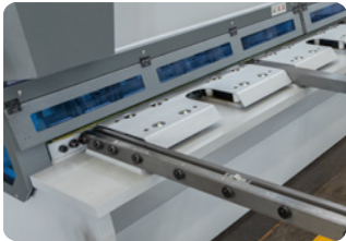
Square support arm with 1000mm scale and flip
